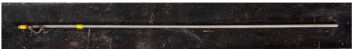
Fig 11 One of the new sediment monitoring pins; 1m long x 10mm diameter stainless steel rod
