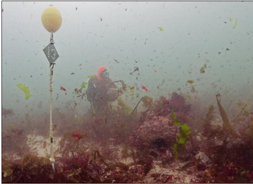
Fig 7 One of the new station markers installed by CISMAS in September 2025. Note the station number (13) drilled into the stainless-steel plate.
