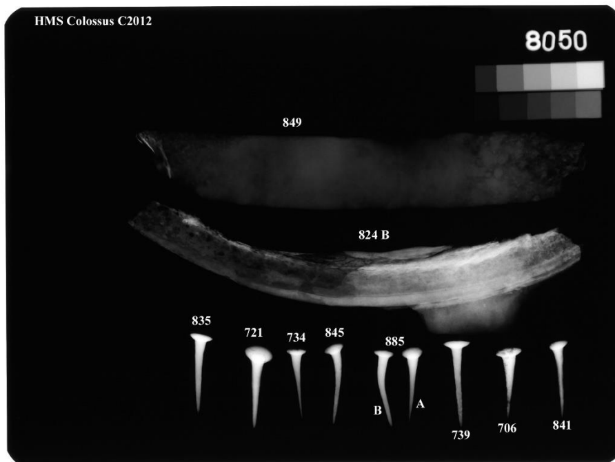
Fig 40: X-ray of all copper alloy artefacts, 2012.
