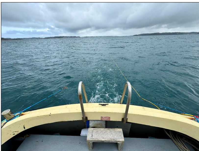
Fig 14 View from the stern of the survey vessel. The magnetometer is on the port side and the side-scan sonar on the starboard side
