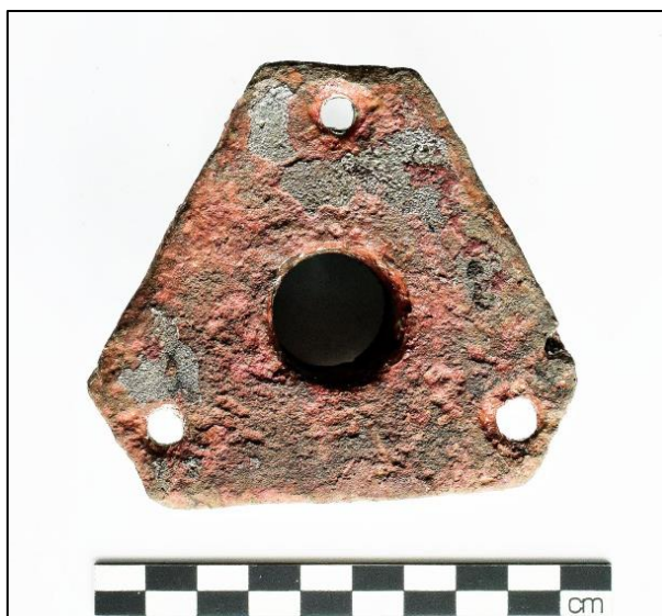
Fig 50 - Triangular copper alloy coak (F22) found on the Wheel Wreck in 2018
