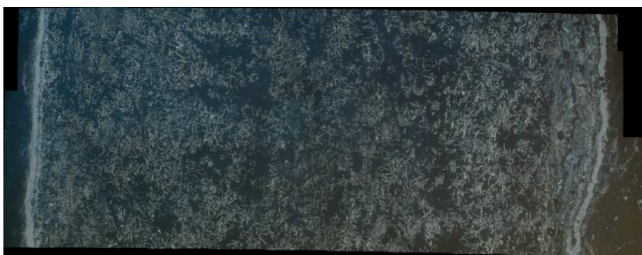
Fig. 3: Photomacrograph showing the totally corroded nature – resembling a photographic negative – of the original cast iron from which the engine cylinder wall was cast (magnification approx x5).
