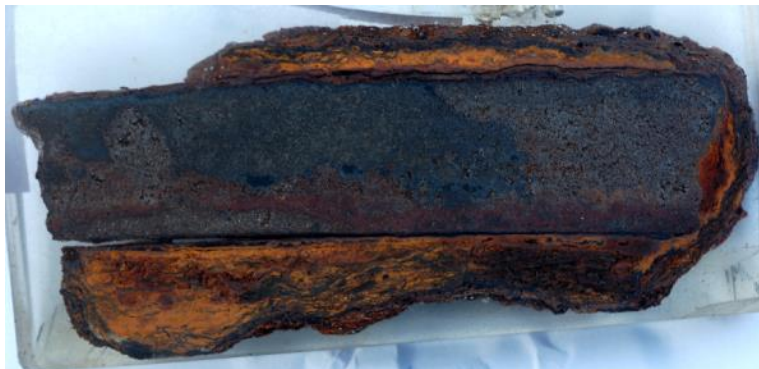
Fig. 2: Polished section through a fragment of the steam engine cylinder (the cylinder itself is 1.08m in diameter). The cast iron of the cylinder wall is 88mm long, and is the roughly rectangular piece in the centre of the section - view almost totally mineralised, much of the dissolved iron having re-precipitated to form the rusty brown corrosion crust on the outside (approximately life size).
