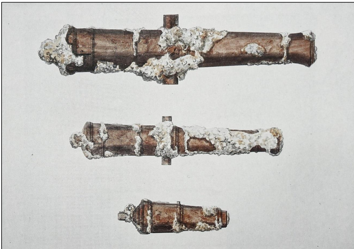
Fig 17 – Deane’s drawing of guns recovered from Colossus. They are probably an 18lb Armstrong (upper gun deck), 9lb Armstrong (quarter deck/forecastle) and a Carronade (Bevan, 1996). It is interesting to note how much iron corrosion concretion had accumulated on the guns in just 35 years.
