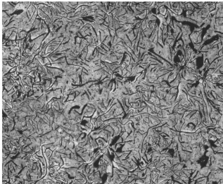
Fig. 6: Detailed view of part of the same structure of the cast iron Newcomen engine cylinder seen in fig. 4. A generally grey cast iron structure of black graphite flakes is visible against a mainly dark grey steel matrix with some pale (ferritic) iron areas also visible (etched 2% nital, field of view 2.5mm, magnification as seen here approximately x50).
