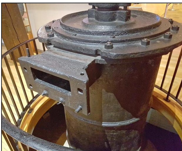
Fig 35 A 33 inch engine cylinder on display in the Science Museum, London. This engine was known as 'Old Bess' and was built by Boulton and Watt in 1777. It was used to pump water to drive a water wheel in their Soho works in Birmingham. Note the rectangular steam port similar to that found on the Wheel Wreck cylinder fragment (C1).
