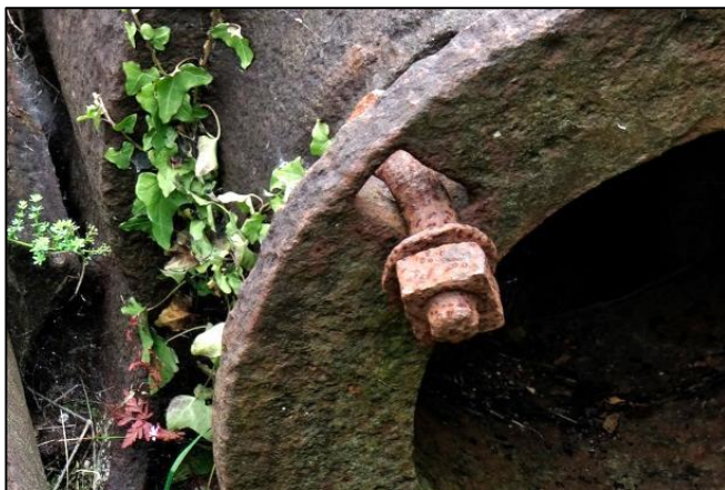
Fig 37 Detail of the square flange holes, round bolts with square heads and round washers common on Cornish pitwork in the 18 th and early 19 th century. This example is at East Pool Mine, Taylor's Shaft near Redruth.
