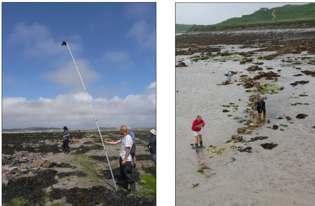
Fig 10 Camera mounted on telescopic levelling staff (left) and an example of an overhead view obtained using the system (right).
