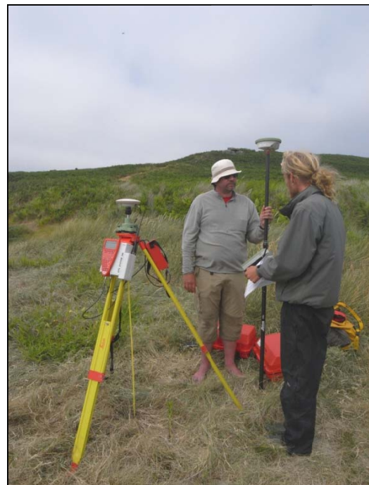
Fig 8 The Leica 1200 series SmartRover (right) and the Leica 500 series reference station (left).
