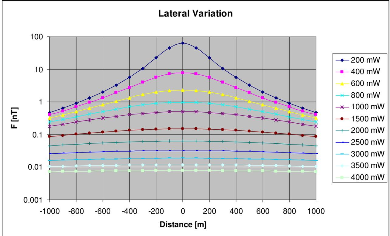
Fig 28 Change of estimated total amplitude with lateral distance from target for different depths
