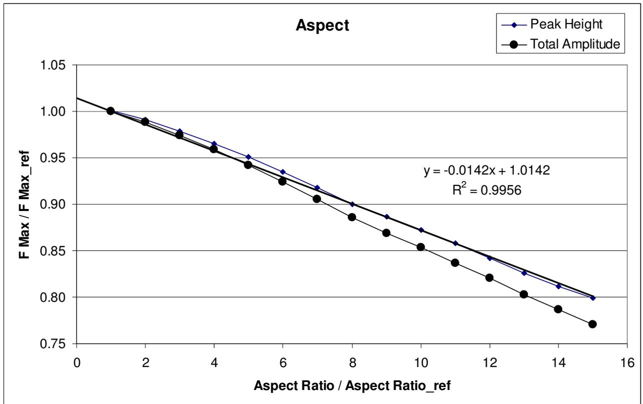
Fig 20 Decrease of anomaly with aspect ratio (ie elongation) for the empty model
