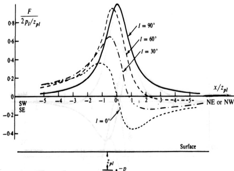
Fig 51 The anomaly shape generated by the same target at different latitudes
