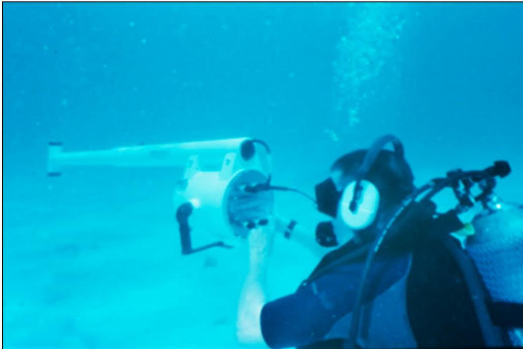
*Figure 43 Diver held caesium magnetometer*
