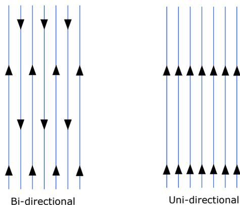
Fig 44 (above left) and Fig 45 (above right) Bi-directional and uni-directional runlines, with survey vessel heading indicated by directional arrows
