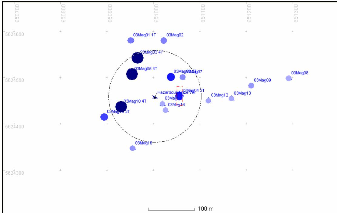
Fig 61 Plan of anomalies where circle diameter indicates estimated mass relative to other anomalies
