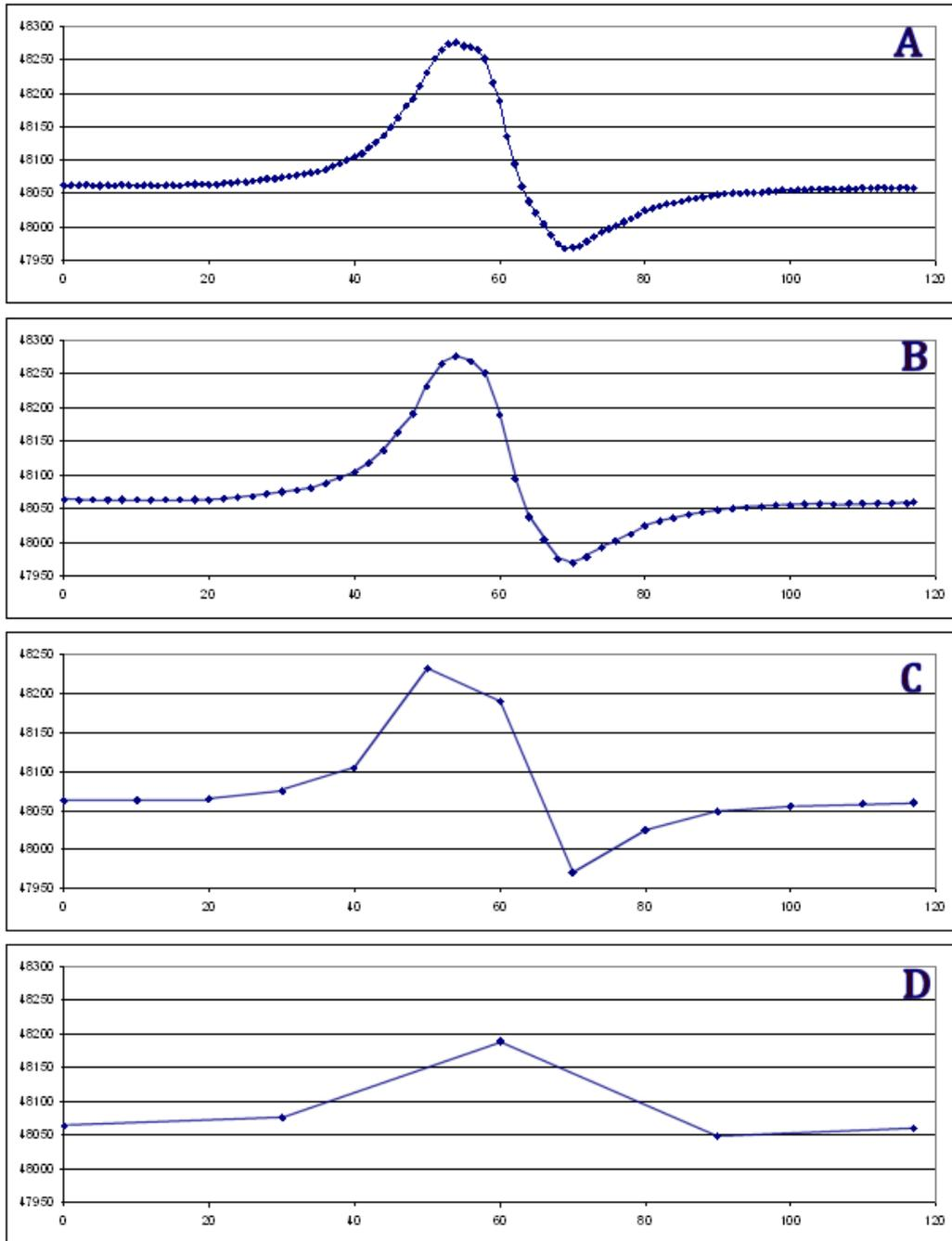
Fig 6 The effects of sampling the same anomaly at 10 Hz, 5 Hz, 1 Hz and 0.3 Hz. X axis in seconds
