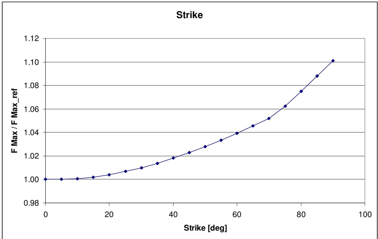
Fig 24 Increase of peak height with strike for dense model
