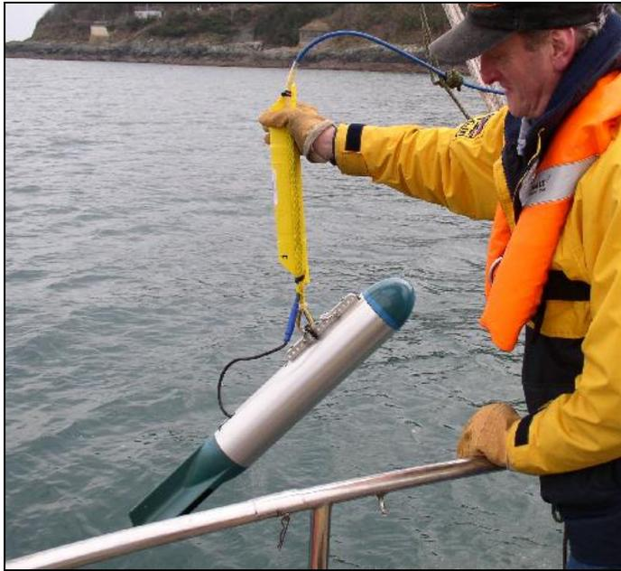
*Fig 42 Towfish with yellow USBL transponder beacon*
