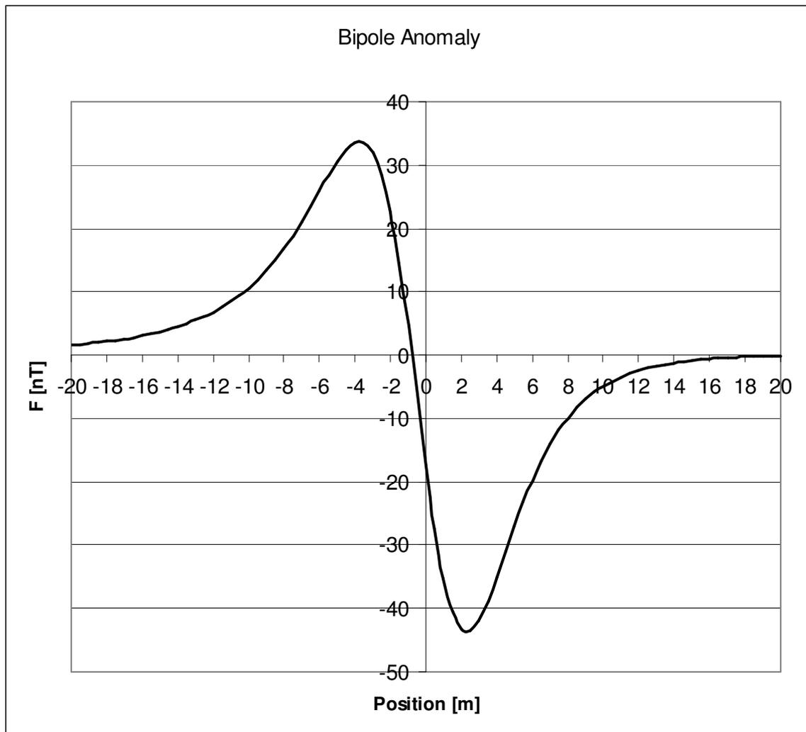
Fig 13 Bipole anomaly for the dense reference model (Figure 13) passing from south to north (left to right) with the centre of the target at position 0 m
