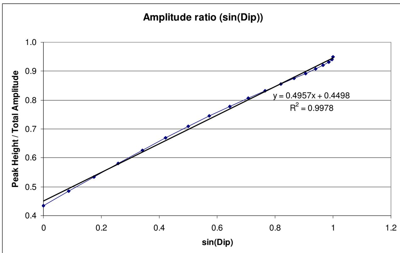
Fig 23 Change of the amplitude ratio in a bipole model with varying dip angles for the dense model
