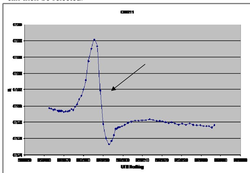
Fig 54 An example of a series plot from the 2005 Colossus Debris Field Survey. The magnetic field strength has been plotted against the UTM northings – the survey lines were essentially north-south. This shows a dipole target of 13 nT total deflection. The arrow shows the data point chosen to take the anomaly's position from
