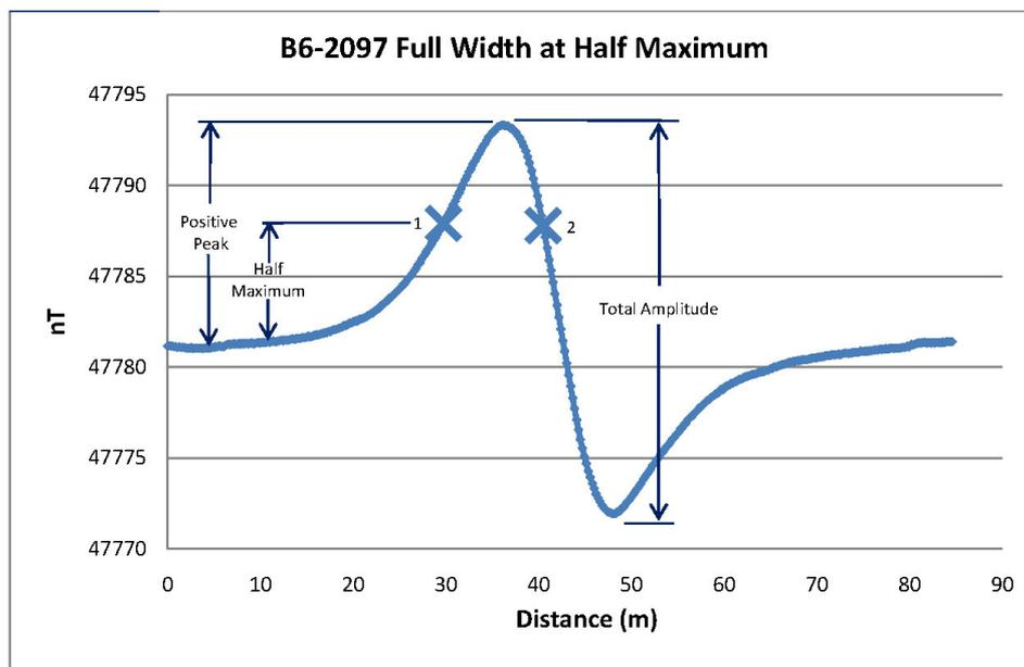
Fig 34 The distance between points 1 and 2 on the time series plot of the magnetometer signal is used to calculate an approximation of the slant range between the towfish and the target
