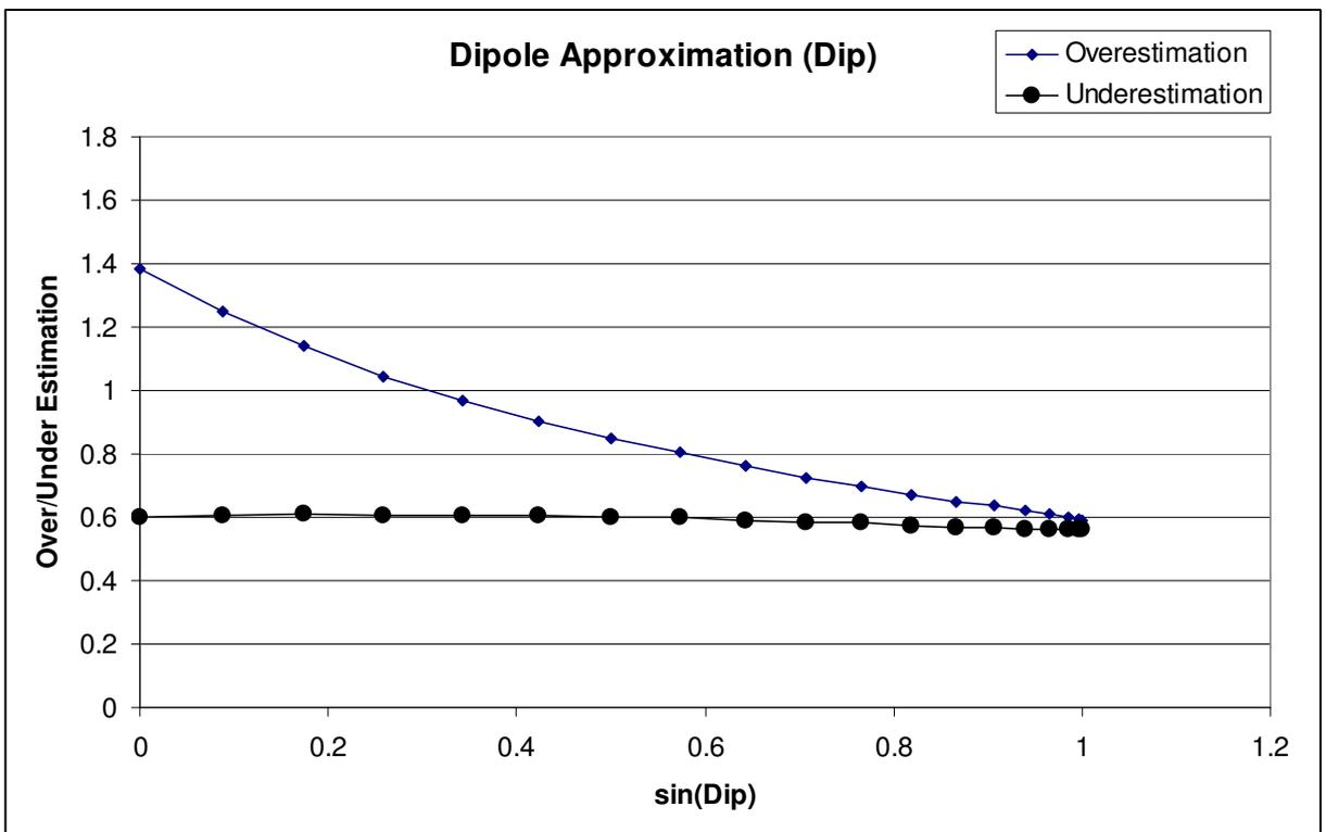
Fig 26 the dipole approximation over- and underestimates the peak height and underestimates the total amplitude. The dependency on the dip of the target (here for the dense model) is very different for the two estimates
