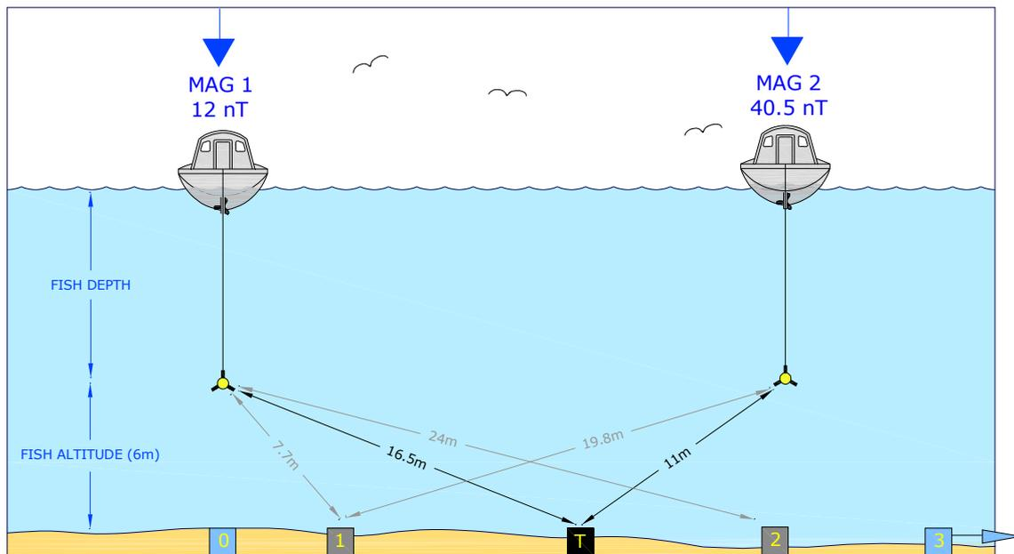
Fig 52 Illustration of the method used to estimate target position where the same target was detected on two adjacent run lines
