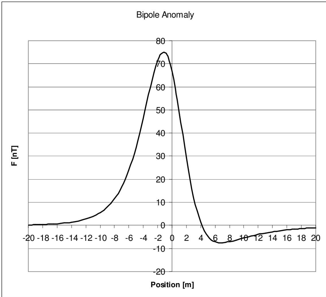
Fig 22 Bipole anomaly for a  $70^\circ$  dip angle of the dense model
