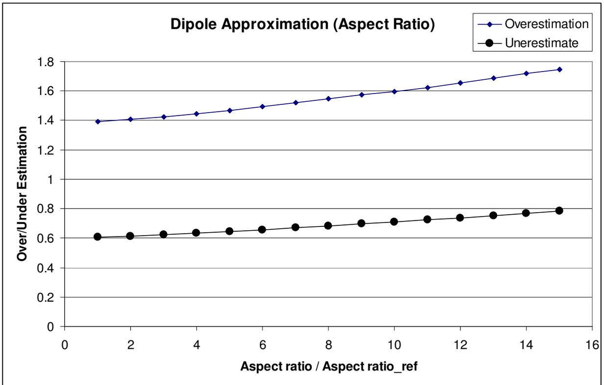
Fig 25 The dipole approximation overestimates the peak height and underestimates the total amplitude. Both show similar dependency on the aspect ratio for the empty model
