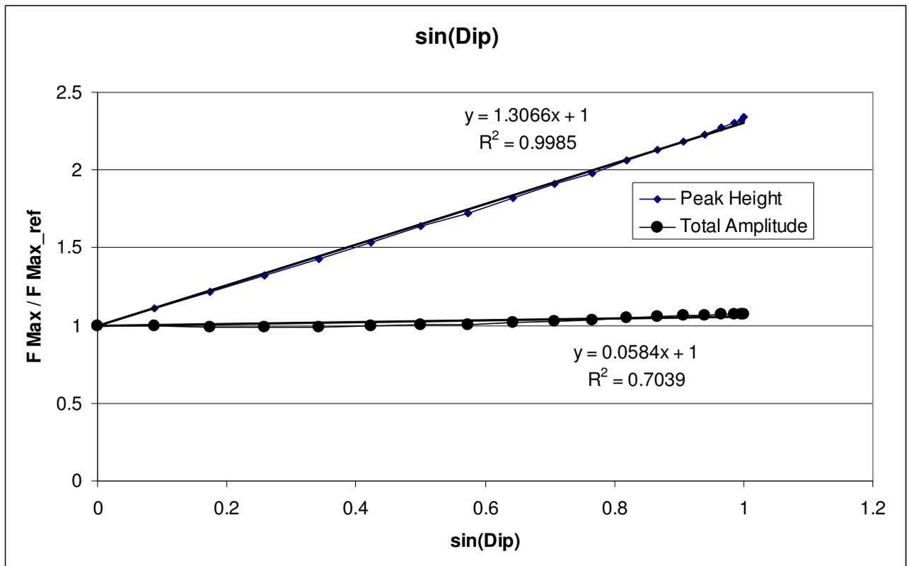
Fig 21 Increase of anomaly with dip for dense model
