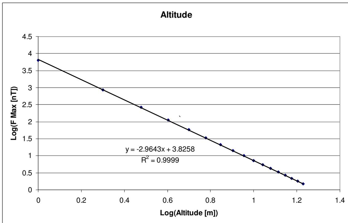
Fig 14 Double logarithmic plot of the decrease of the peak height with increasing altitude for the dense model. The slope of -2.96 is very close to the value of -3 for a dipole approximation
