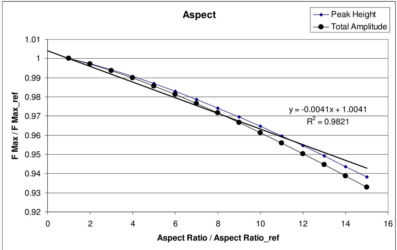
Fig 19 Decrease of anomaly with aspect ratio (ie elongation) for the dense model
