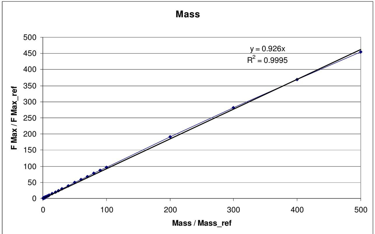
Fig 17 Nearly proportional increase of anomaly with mass for the dense model
