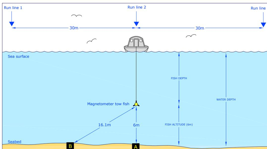
Fig 39 Showing the effect of run line spacing on magnetometer to target distance
