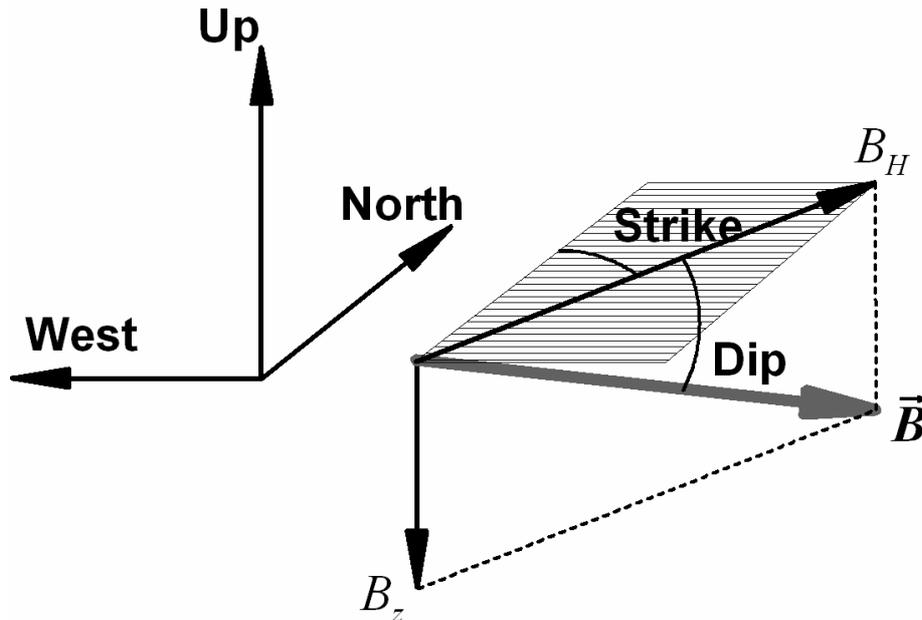
Fig 11 Angles of the vector anomaly  $\vec{B}$
