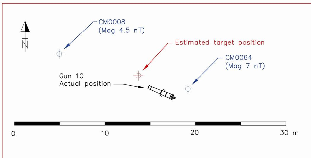
Fig 55 An example of target position estimation using data from two adjacent run lines
