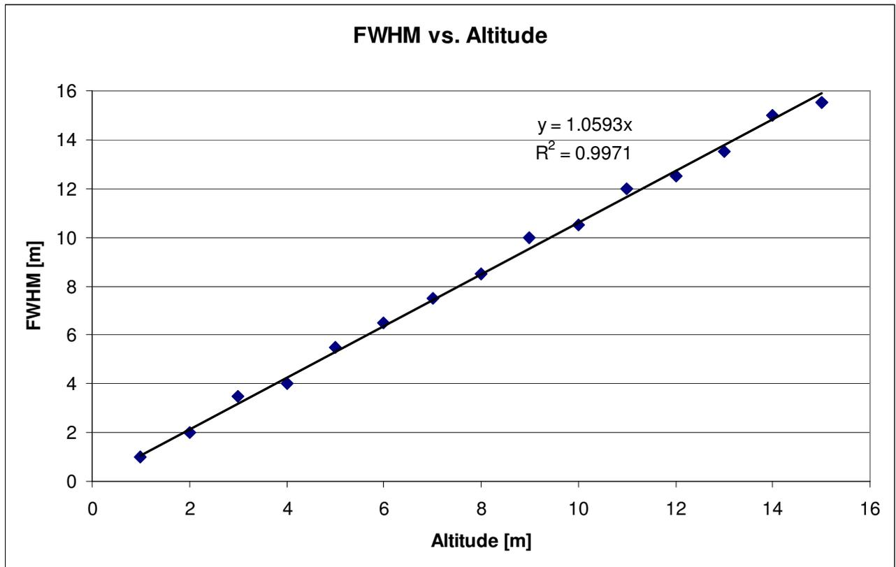
Fig 15 Change of the positive peak's width with altitude. The width is measured at half the peak height (Full Width at Half Maximum). The linear dependency has a slope slightly larger than 1
