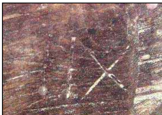
E8 Detail of the eastern knee on the orlop deck, showing possible builders' mark 'IIX'. Photograph by Robin Witheridge.
