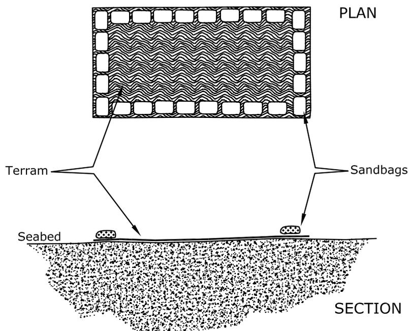
*The Terram mat (V1) as deployed in these trials – note the use of sandbags to anchor the mat.*
