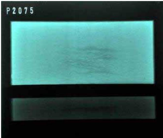
*Fig 36 X-radiograph of oak test block protected by Terram 4000 (length of exposure 24 months). No terredo attack*
