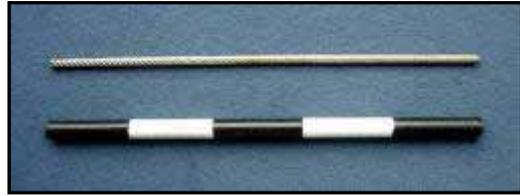
The amount of monitoring pin exposed was measured at each data retrieval visit to the site. This was achieved by placing a 1m bar on the seabed adjacent to the pin and measuring the distance from the top of the pin to the bottom of the bar. This method of measurement avoided distorting the measurements by discounting any localised scouring around the pin itself.
