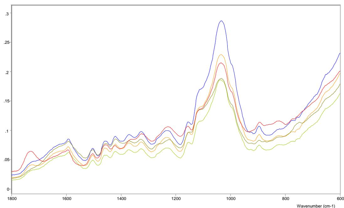
*Fig 62 FT-IR spectra of oak samples (24 month exposure)*
