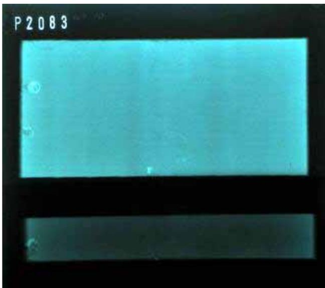
*Fig 43 X-radiography of pine wood block protected by mesh (after 24 months). Slight attack*
