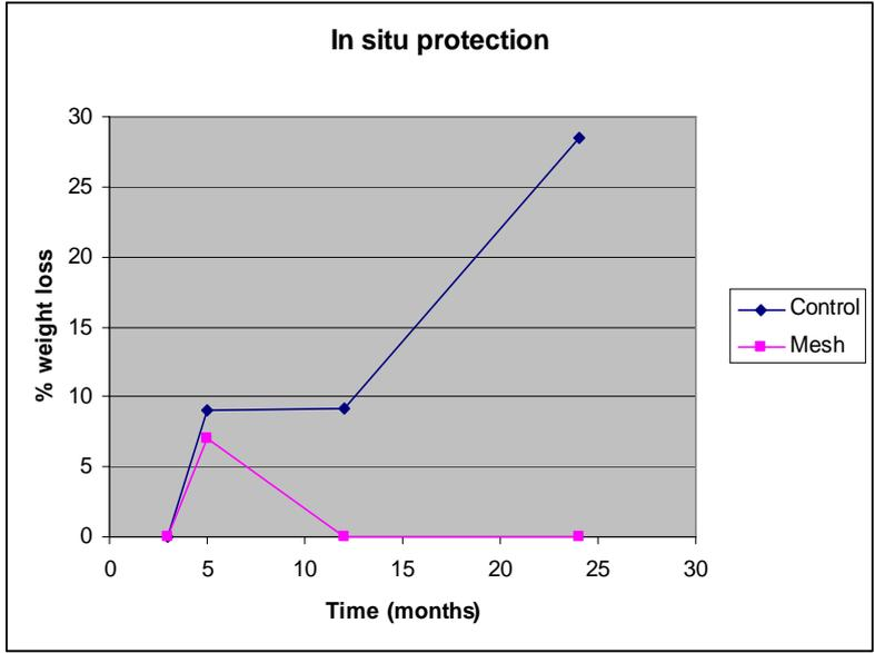
Fig 53 % weight loss of Oak comparing Mesh with the Control sample
