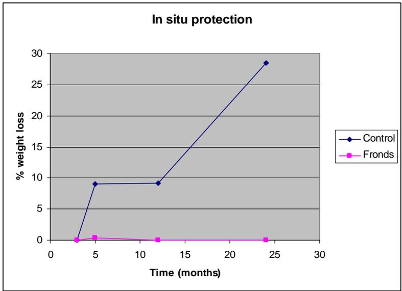
Fig 54 % weight loss of Oak comparing Fronds with the Control sample
