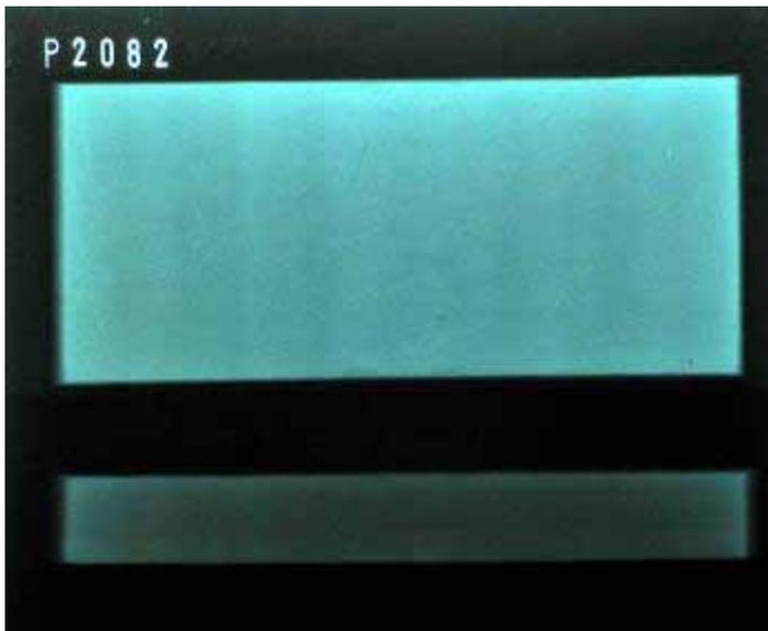
*Fig 37 X-radiography of Pine test block protected by Terram 4000 (length of exposure 24 months). No Terredo attack*
