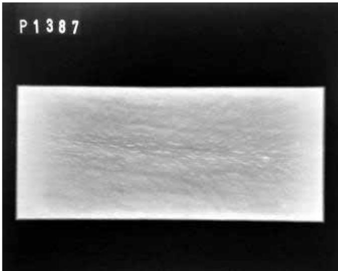
*Fig 44 X-radiograph of oak test block protected by frond matting (after 5 months). No attack*
