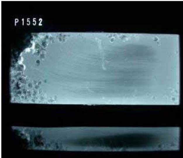
*Fig 28 X-radiograph of Oak sample after 12 months exposure (no protection). Severe attack*
