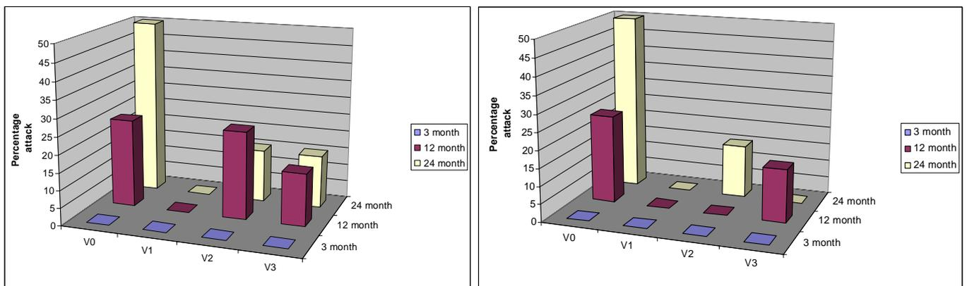
Fig 25 Charts illustrating the approximate percentage attack for the test blocks in each of the trial areas V0 – V3. Note that the only trial area blocks to show no attack are those from V1, the Terram 4000.
