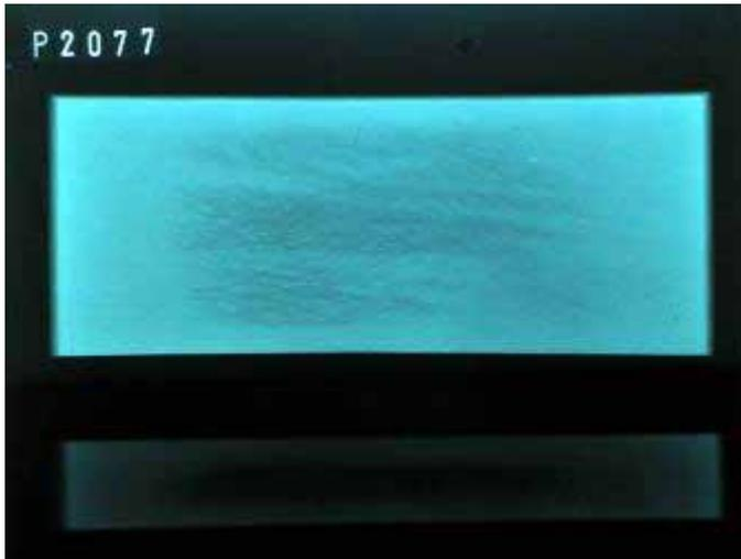
*Fig 48 X-radiograph of oak test block protected by frond matting (after 24 months). No attack*
