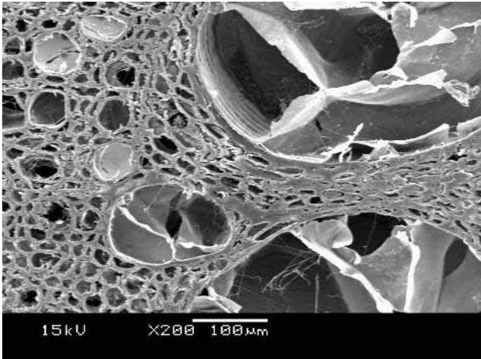
*Fig 16 Scanning electron micrograph of oak sample protected by Terram 4000. No evidence of bacterial and fungal decay (24 month exposure).*
