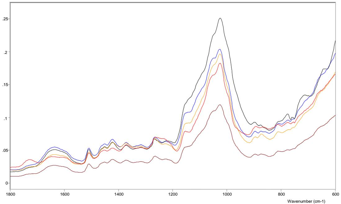
Fig 63 FT-IR spectra of pine samples (24 month exposure)
