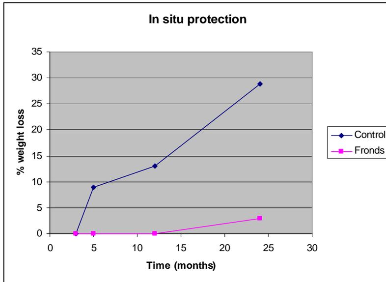
Fig 58 % weight loss of Pine comparing Fronds (V3) with the Control sample (V0)
