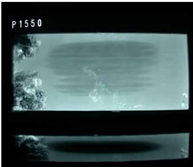
*Fig 41 X-radiography of Pine wood block protected by mesh (after 12 months). Moderate attack*
