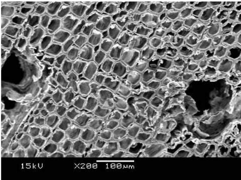
*Fig 22 Scanning electron micrograph of pine sample protected by a frond mat (24 months exposure). Early signs of decay by erosion bacteria.*
