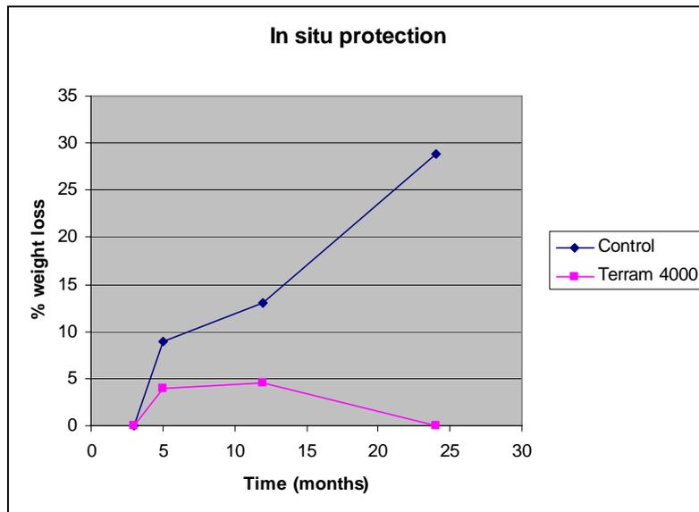
Fig 56 % weight loss of Pine comparing Terram 4000 (V1) with the Control sample (V0)
