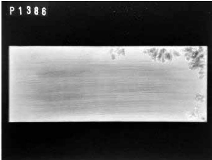
*Fig 38 X-radiography of Oak wood block protected by mesh (after 5 months). Slight attack*
