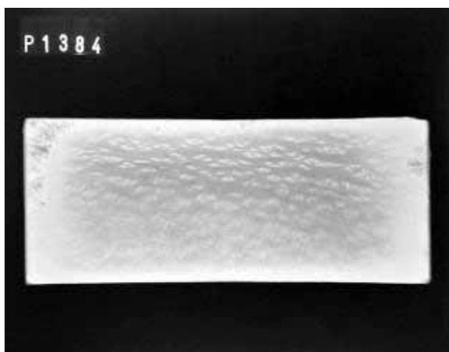
Fig 26 X-radiograph of Oak after 5 months exposure (no protection). Slight attack
