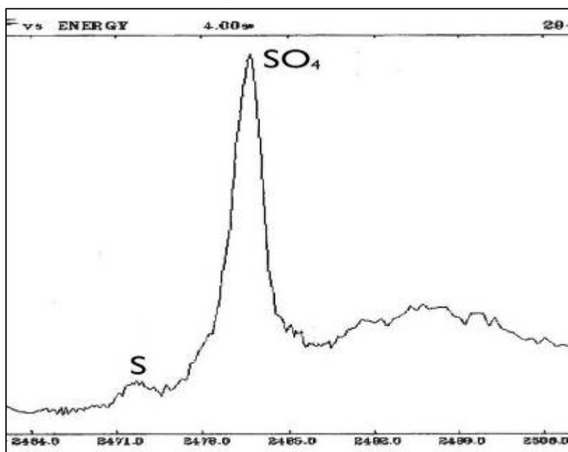
Fig 60 K-edge XANES spectrum of oak sample protected by Terram 4000.
