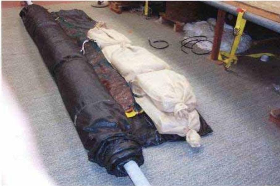
**5. Simulated Sand / Gravel Bags laid over the Inner Edge Membrane**
