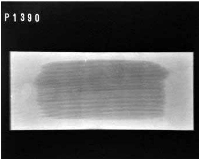
*Fig 39 X-radiography of Pine wood block protected by mesh (after 5 months). No terredo attack*
