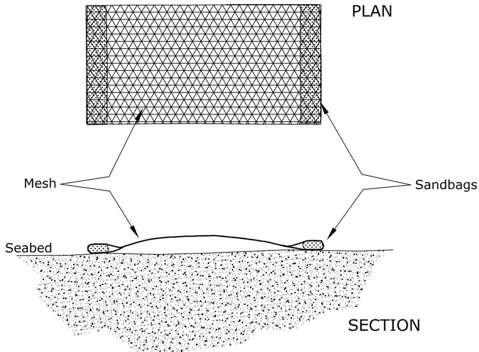
*The mesh system (V2) as deployed in these trials – note the use of sandbags instead of chain to anchor the mat..*
