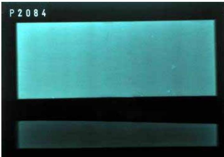
*Fig 49 X-radiograph of pine wood block protected by frond matting (length of exposure 24 months). Slight attack*
