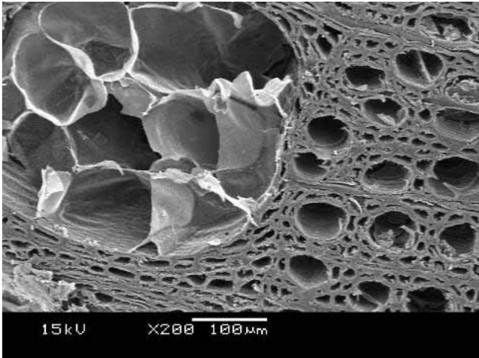
*Fig 18 Scanning electron micrograph of oak sample protected by a frond mat (24 months exposure). No evidence of bacterial or fungal decay.*
