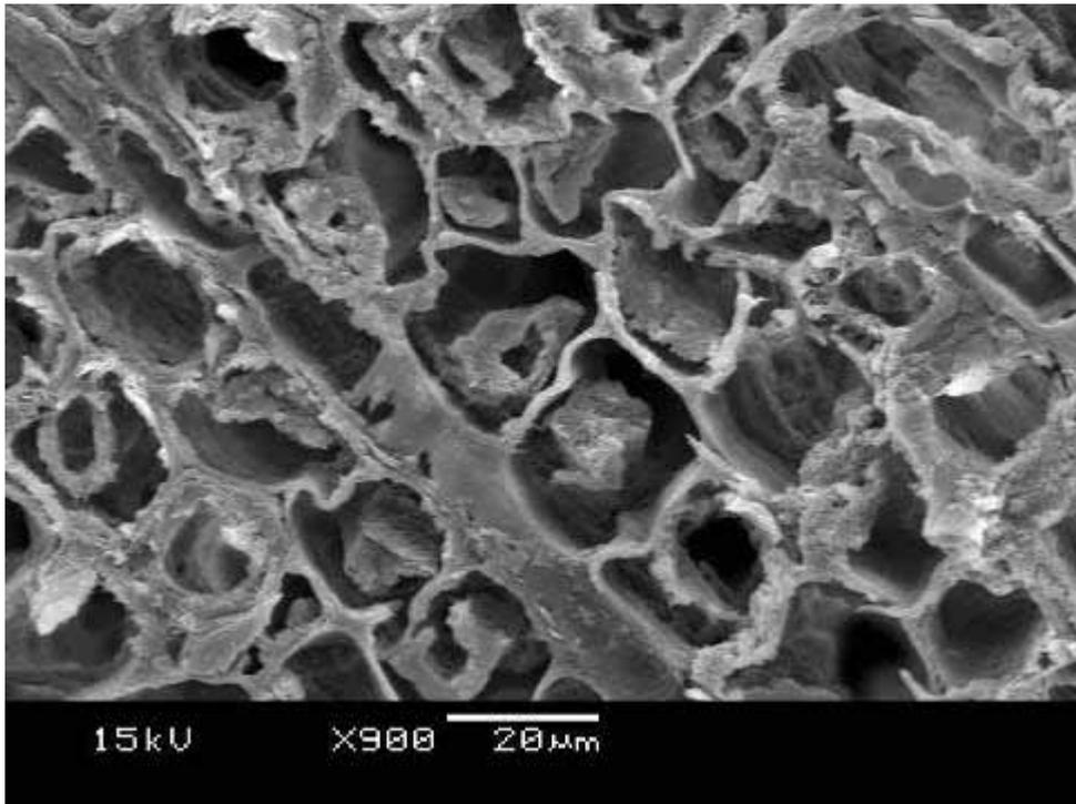
*Fig 19 Scanning electron micrograph of pine sample (control-24 month exposure). Note erosion to secondary wall layers.*
