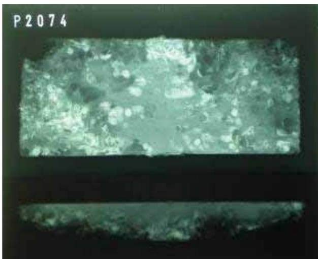
*Fig 30 X-radiograph of oak after 24 months exposure (no protection). Failure*
