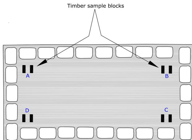
Position of the timber sample blocks under the trial mats.
