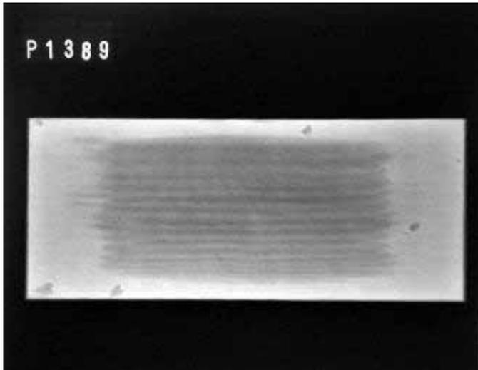
*Fig 33 X-radiograph of Pine after 5 months exposure protected by Terram 4000. Slight attack*
