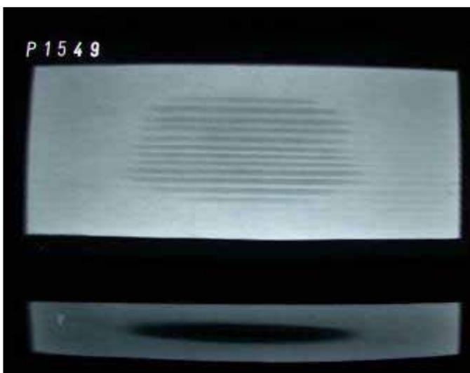
*Fig 35 X-radiograph of Pine after 12 months exposure protected by Terram 4000. No Terredo attack*
