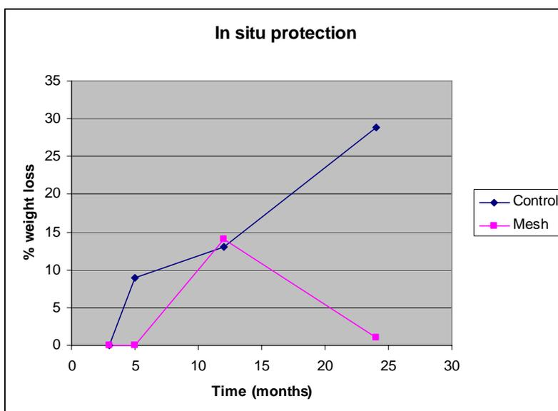
Fig 57 % weight loss of Pine comparing Mesh (V2) with the Control sample (V0)
