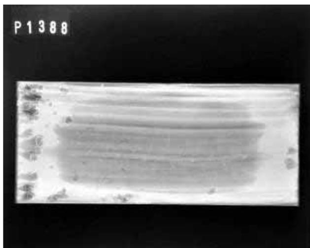
Fig 27 X-radiograph of Pine after 5 months exposure (no protection). Moderate attack
