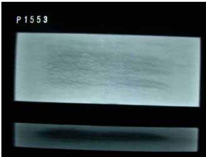
*Fig 34 X-radiograph of Oak after 12 months exposure protected by Terram 4000. No Terredo attack*
