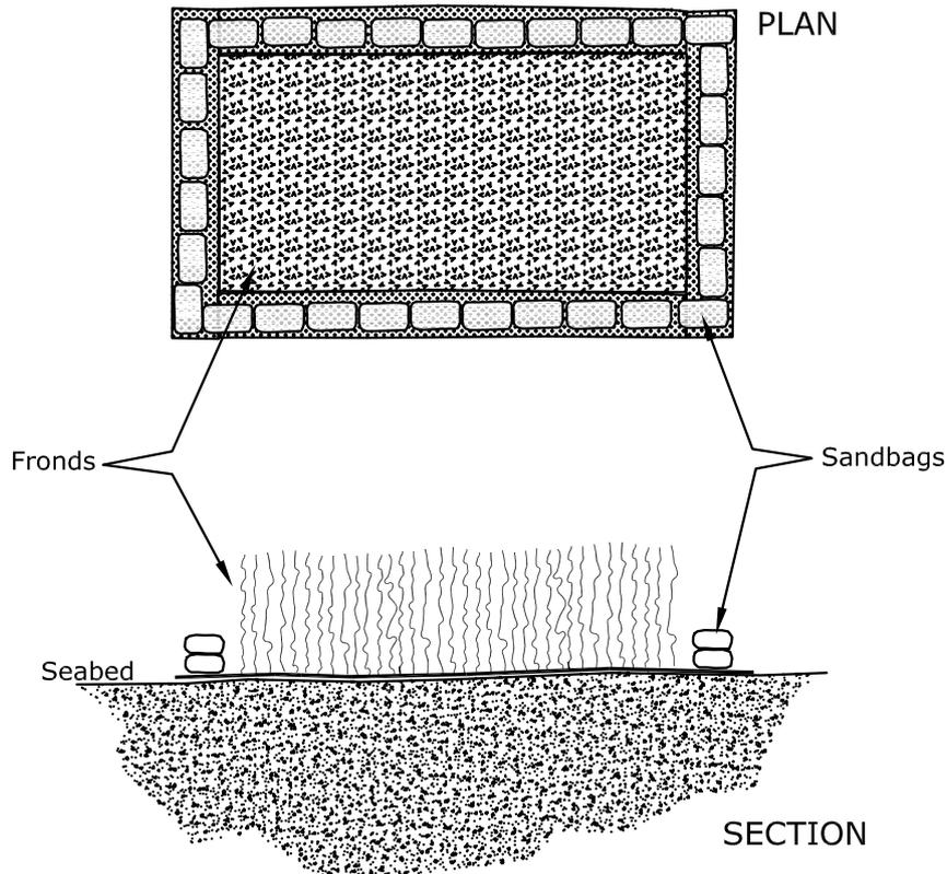
*The Seabed Scour Systems frond mat (V3) as deployed in these trials – note the double layer of sandbags used to anchor the mat.*
