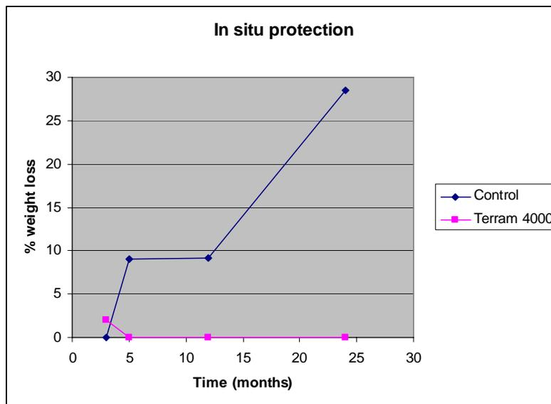
Fig 52 % weight loss of Oak comparing Terram 4000 with the Control sample
