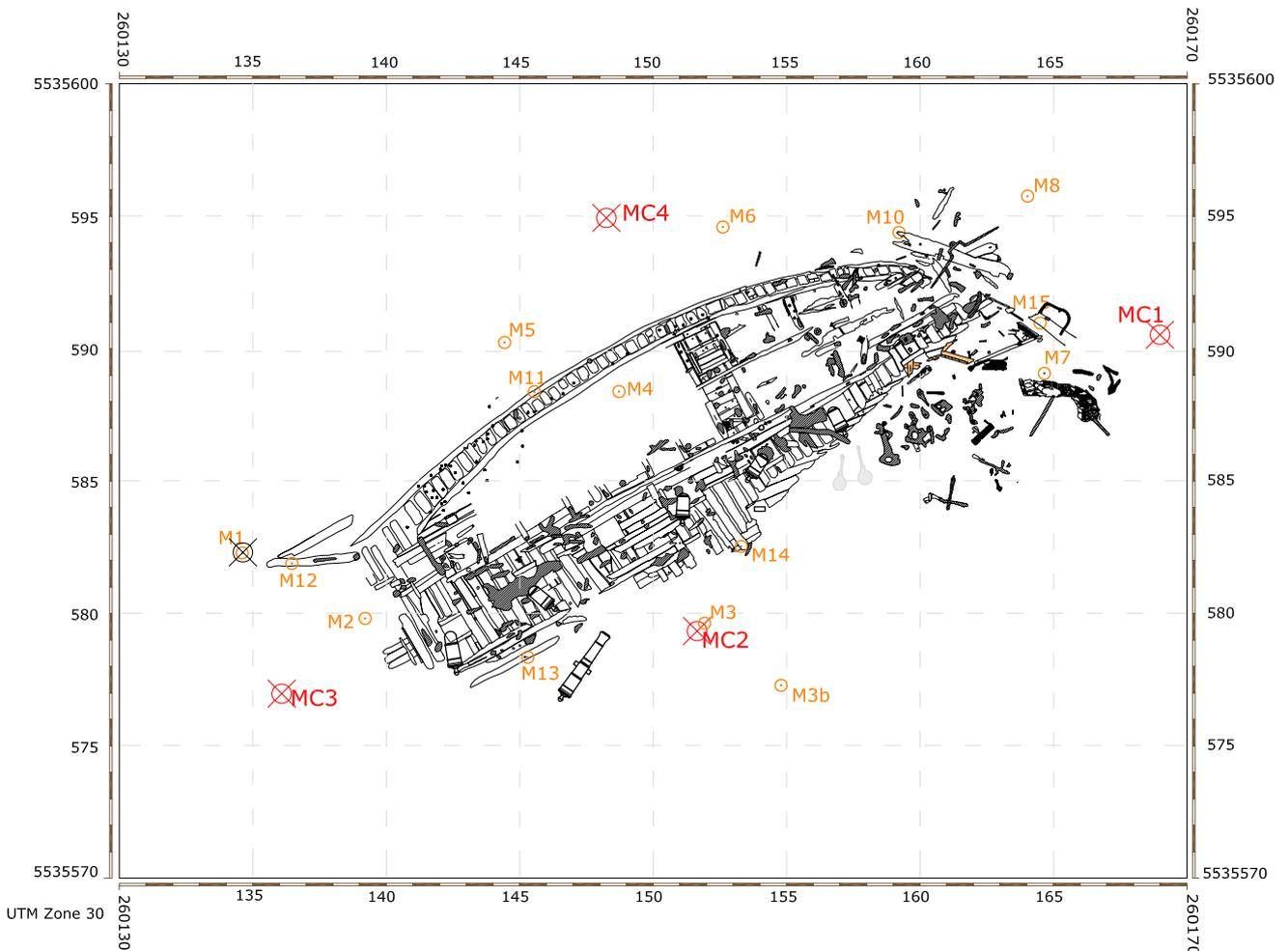
Fig 3 Plan showing the location of the sediment level monitoring pins
