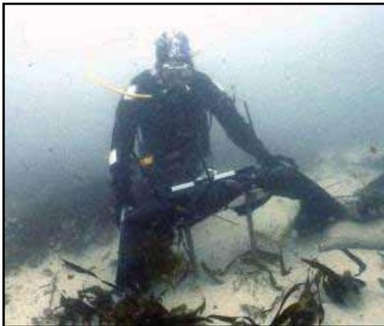
*Fitting the butyl cover to the data logger*
