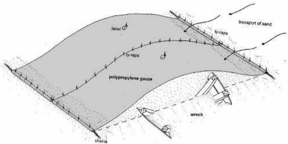
*The mesh protection system as deployed on the BZN 10 and Darsser Cog sites by Martijn Manders – note the use of chain to anchor the mat.*
