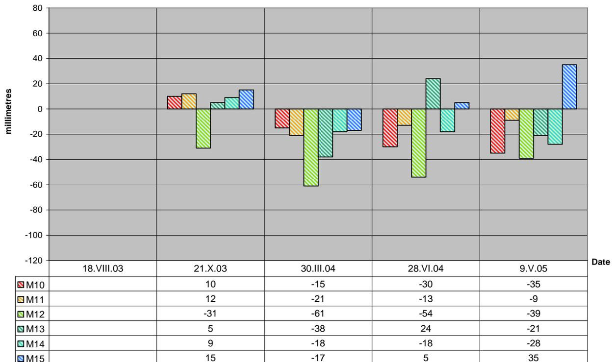
Fig 11 Seabed levels relative to those in August 2003 at monitor points M10 –M15
