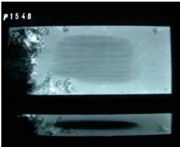
*Fig 29 X-radiography of Pine after 12 months Exposure (no protection). Severe attack*
