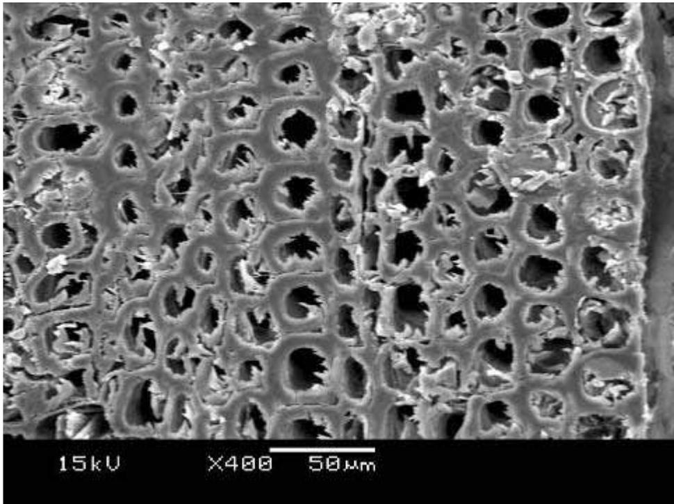
*Fig 21 Scanning electron micrograph of pine sample protected by a mesh netting (24 months exposure). Note decay of some cells.*
