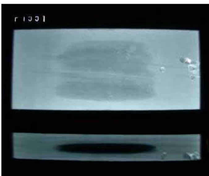
*Fig 47 X-radiograph of Pine test block protected by frond matting (after 12 months). Slight attack*
