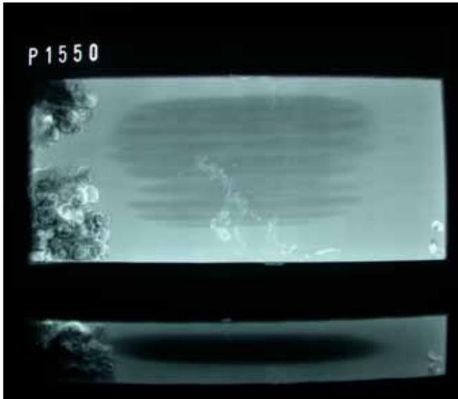
*Fig 40 X-radiography of Oak wood block protected by mesh (after 12 months). Moderate attack*
