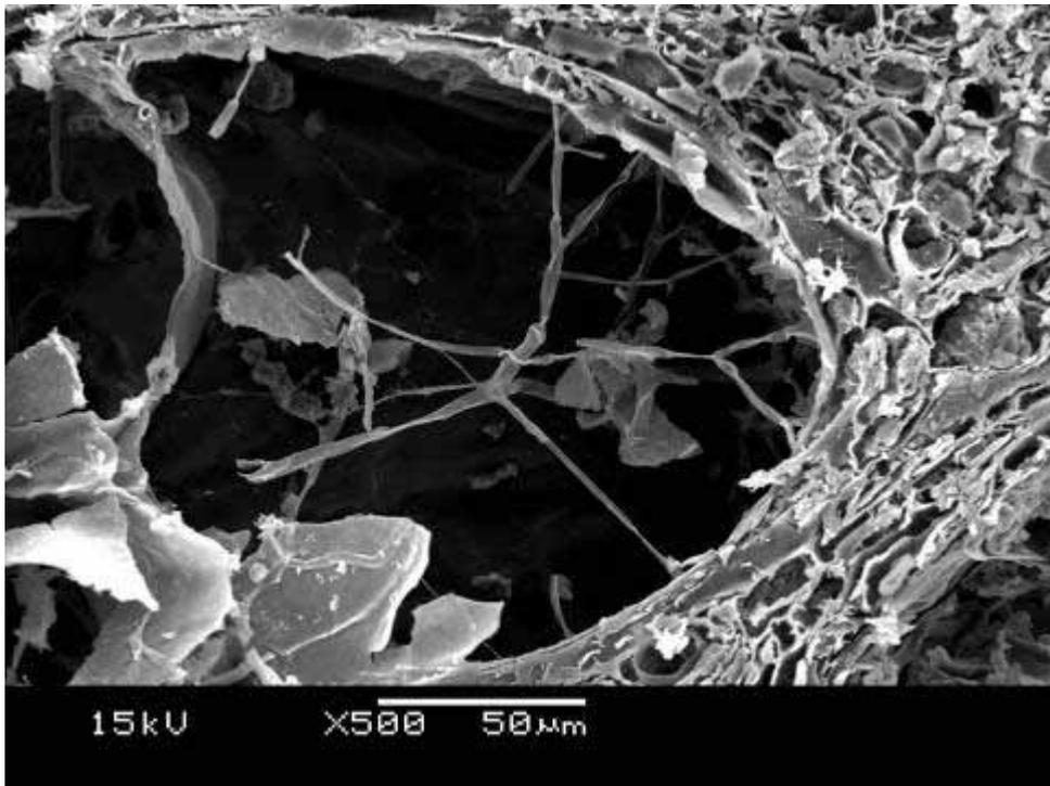
*Fig 15 Scanning electron micrograph of oak sample (control) exposed for a period of 24 months. Bacterial erosion of secondary wall layers very advanced. Fungal hyphae present in vessel.*
