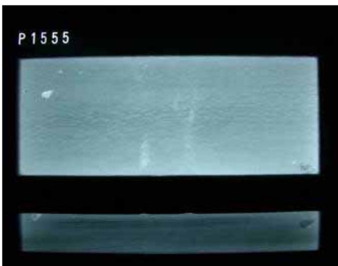
*Fig 46 X-radiograph of Oak test block protected by frond matting (after 12 months). Slight attack*
