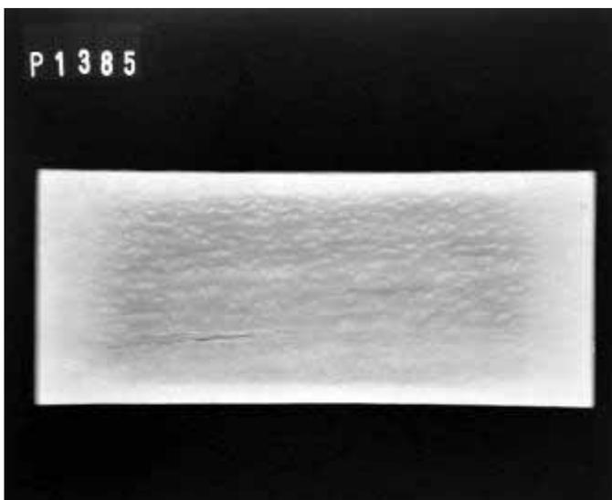
*Fig 32 X-radiograph of Oak after 5 months exposure protected by Terram 4000. No Terredo attack*
