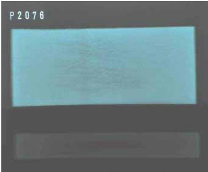
*Fig 42 X-radiography of Oak wood block protected by mesh (after 24 months). No attack.*
