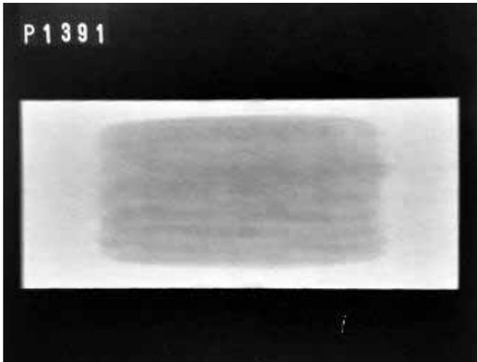
*Fig 45 X-radiograph of Pine test block protected by frond matting (after 5 months). No attack*
