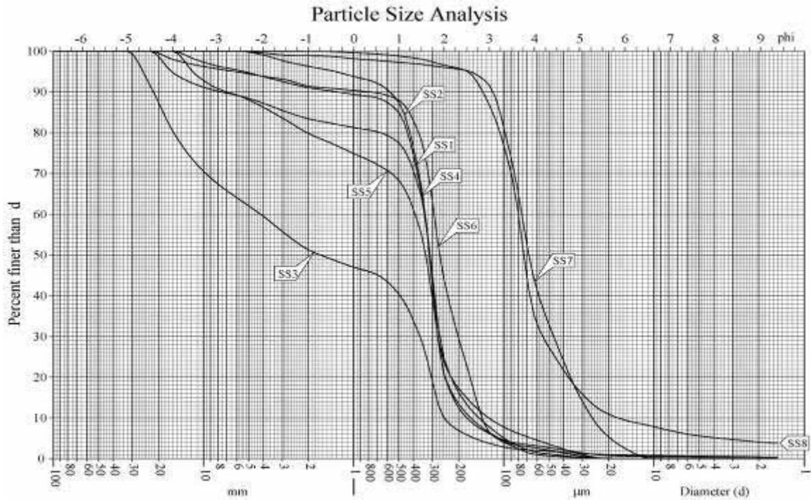
**Figure 2.** Particle size analyses of the Colossus seabed samples.
