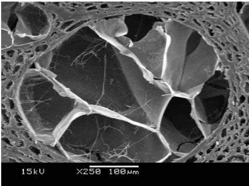
*Fig 17 Scanning electron micrograph of oak sample protected by a mesh system. Cellular structure well preserved, no evidence of bacterial or fungal decay (24 months exposure)*
