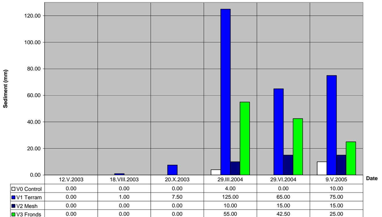
Fig 9 Chart showing the sediment levels in the test areas (mean of the four measurements taken)
