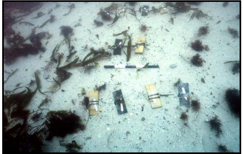
Above : The timber sample blocks on the seabed in the control area V0. Note the steel staples and cable ties used to hold the blocks in position. Scale = 0.5m
