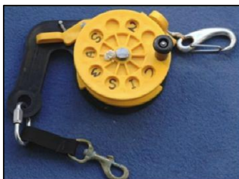
Fig 7. The SMB reel and markings (from the top down) 1m, 3m, 5m and 12m
