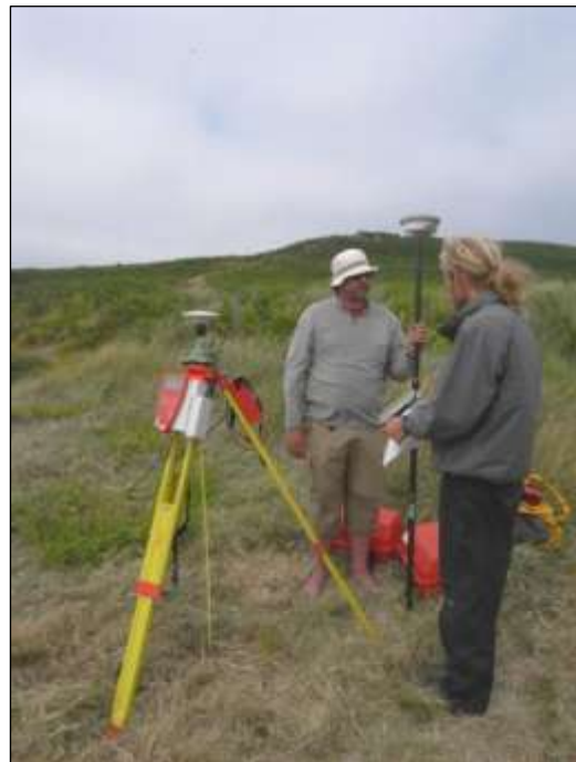
Fig 10 The Leica 1200 series SmartRover (right) and the Leica 500 series reference station (left).
