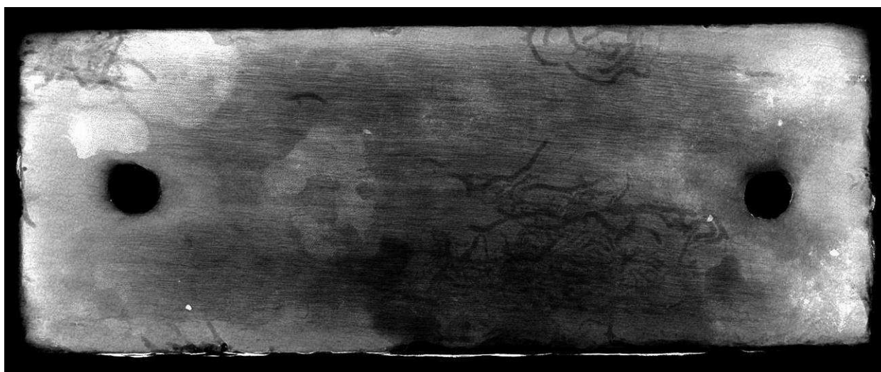
Fig 23 Block 3 showing calcareous surface deposits along bottom edge and three distinct zones of infestation
