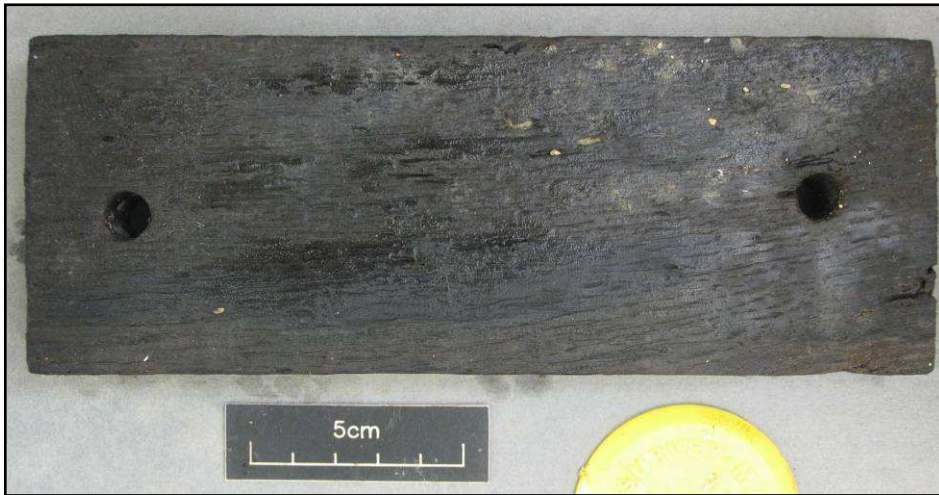
Fig 14 Although block 8 had been buried c.20cm below the seabed surface, and there was no evidence of marine growths on the surface, there was however, evidence of marine borer attack visible on the lower right edge and centre:
