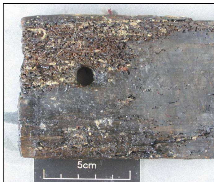
Fig 16 Close-up of decay to block 1. The decay appears to be initiated through the cut ends and sides, in effect proceeding along the vessels and other wood cells. The edges and exposed surfaces of wood blocks 1, 2 and 3 are all deteriorated
