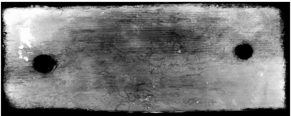
Fig 22 Block 2 calcareous surface deposits and galleries throughout body of wood
