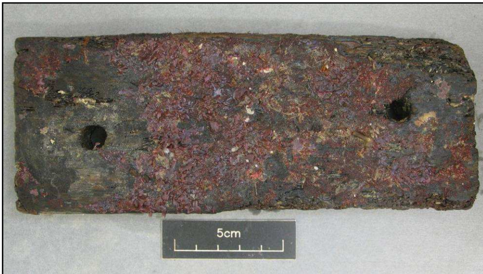
Fig 15 Block 1 showing algal growth on uppermost and exposed surfaces. Blocks 2 and 3 were very similar in appearance. The presence of the yellow plastic number tags has conferred a small degree of protection to the wood surface
