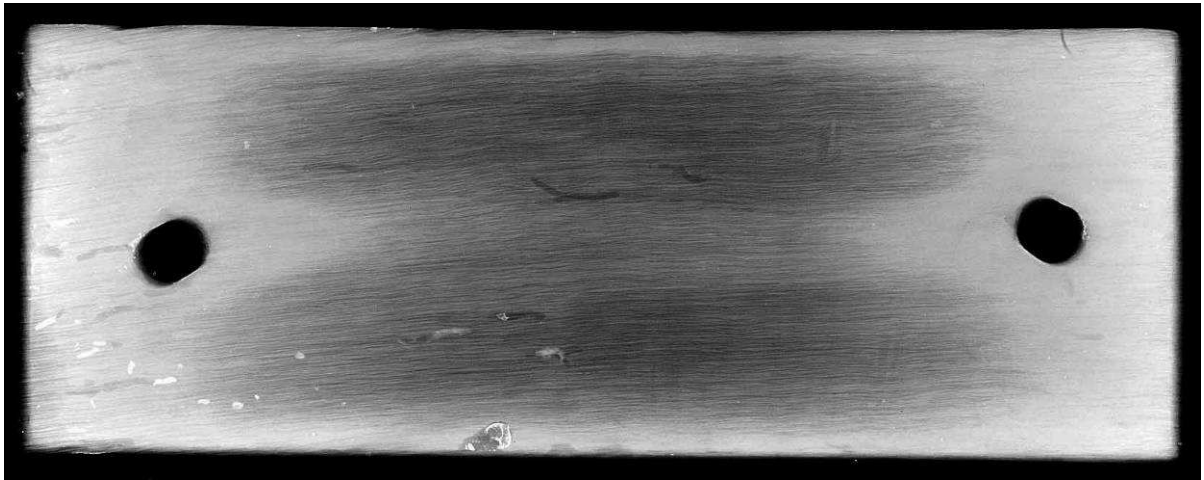
Fig 20 Block 8, slight infestation with galleries to lower left and centre of block
