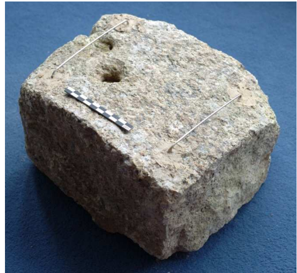
Fig 6 Stainless steel rods set into granite block using drilled holes and polyvinyl resin
