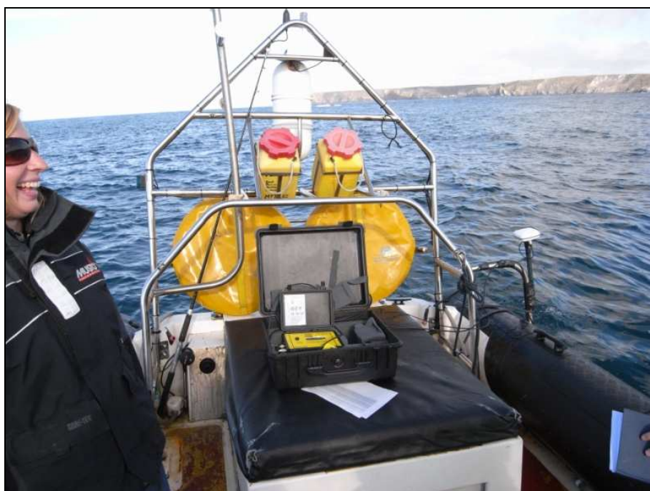
Fig 13 The Ceeducer echo sounder unit onboard the survey vessel Mytilus
