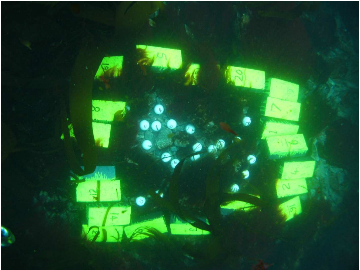
Fig 11 The steatite balls and engineering bricks (20 of each) in place on the seabed
