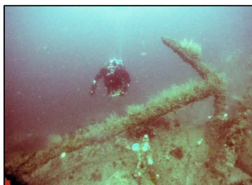
1 One of the Firebrand's four bower anchors – note the missing upper fluke.
