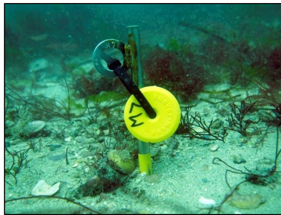
Fig 4. Sediment monitoring pin M7 installed on the seabed (July 2014)
