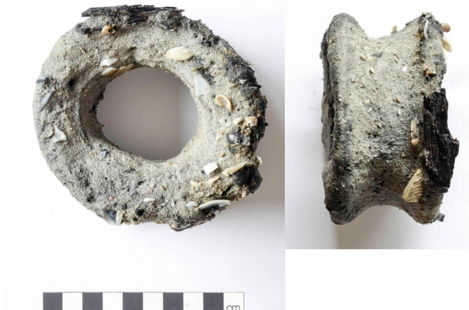
Fig 45 Two views of the iron rope thimble 1301.
